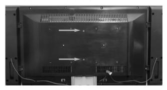
> Now remove the pedestal carefully in the direction of the lower side of the device. You require an additional special profile, in order to be able to use the loudspeakers, if they are situated at the bottom of the device when mounting on a wall. You can purchase this additional profile from your specialised dealer under the following designation and article number.
